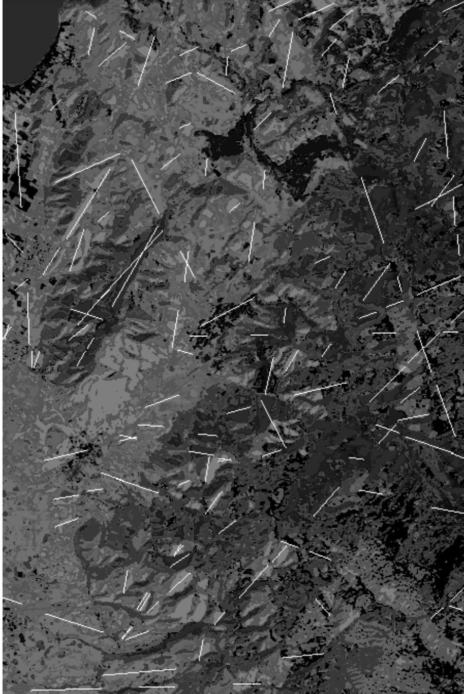
**Fig. 9.** Automatic lineament detection super-imposed on the classification result.
