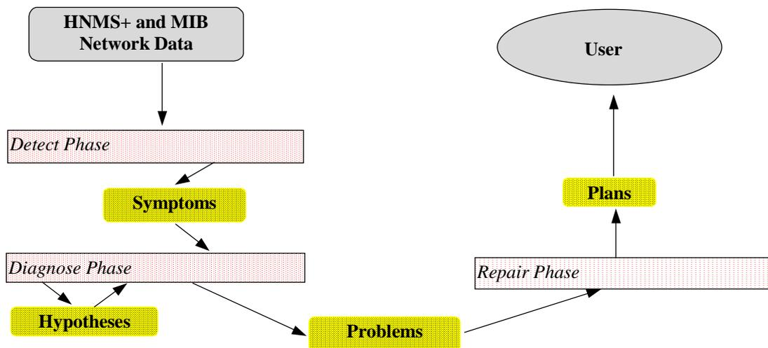
**Figure 3.** Generation of objects during an expert system's operational cycle.
