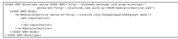
Figure 13. Sample input SOAP message for the cheapest/speediest parcel dispatch request Mediator Service of the courier e-mall.
