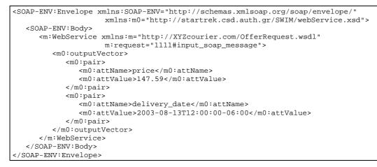
Figure 14. Sample output SOAP message from the parcel delivery offer request Web Service of a courier company.
