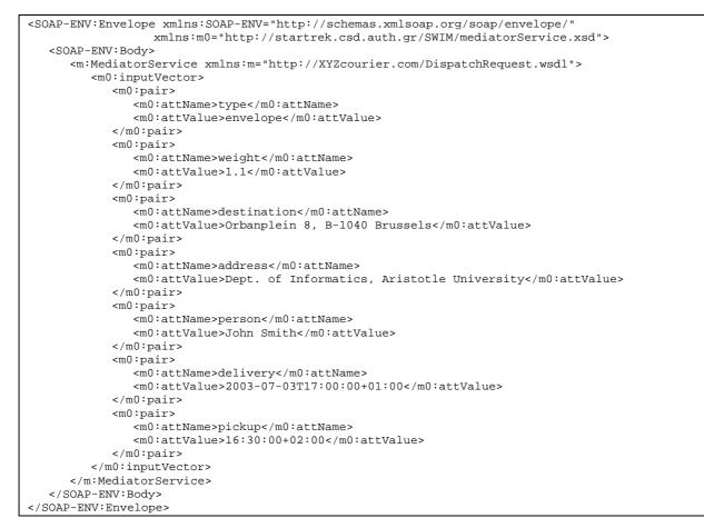
Figure 4. Sample input SOAP message for the parcel dispatch request Mediator Service of the courier.
